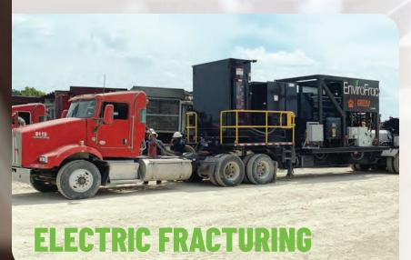
Twin Disc's TA90-7601 e-Frac system consists of a constant-speed electric motor coupled to the transmission, eliminating the need for variable frequency drives and specialized repairs. This configuration allows for a hydraulic synchronous start for effortless power-up and the hydrostatic creep mode provides smooth and safe hydraulic line test.
