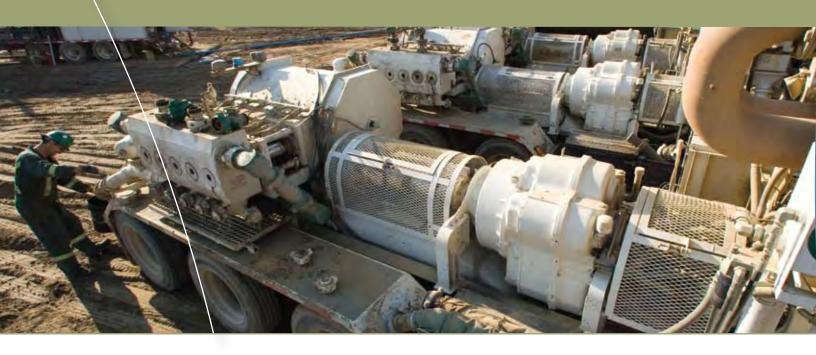
Cover and above: Calfrac Well Services Ltd., a leading service provider of specialized oil field services and hydraulic fracturing to oil and natural gas exploration and production companies, uses Twin Disc 8500 power-shift transmission systems in its fracturing rigs to obtain maximum productivity and reliability for its customers.
