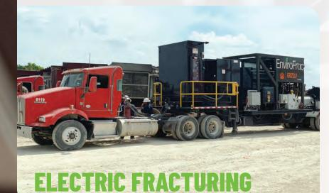
Twin Disc's TA90-7601 e-Frac system consists of a constant-speed electric motor coupled to the transmission, eliminating the need for variable frequency drives and specialized repairs. This configuration allows for a hydraulic synchronous start for effortless power-up and the hydrostatic creep mode provides smooth and safe hydraulic line test.
