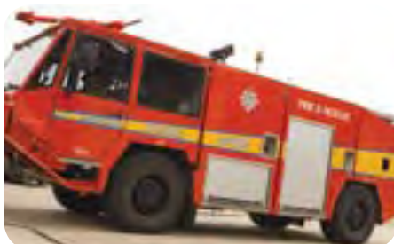
Below: The UK Ministry of Defense recently overhauled this 1999 model ANis UniPower rapid intervention crash fire tender deployed at Mansten Airport (now Kent International) in Kent, England, to incorporate the new Twin Disc TD61-1179 transmission system and TDEC-400 electronic controls.
