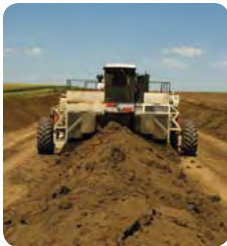
Below: Resource Recovery Systems, Inc.'s KW 614 Composter, shown here traversing a windrow of dried cattle manure, uses a Twin Disc clutch to engage the drum which turns and grinds the manure into a fine compost.
