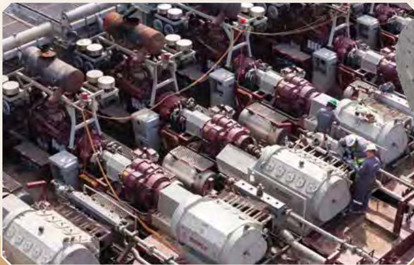
The Twin Disc 7600 oil field transmission offers fracturing operators a durable but lighter hydraulic pumping transmission for mid-range capacity applications.
