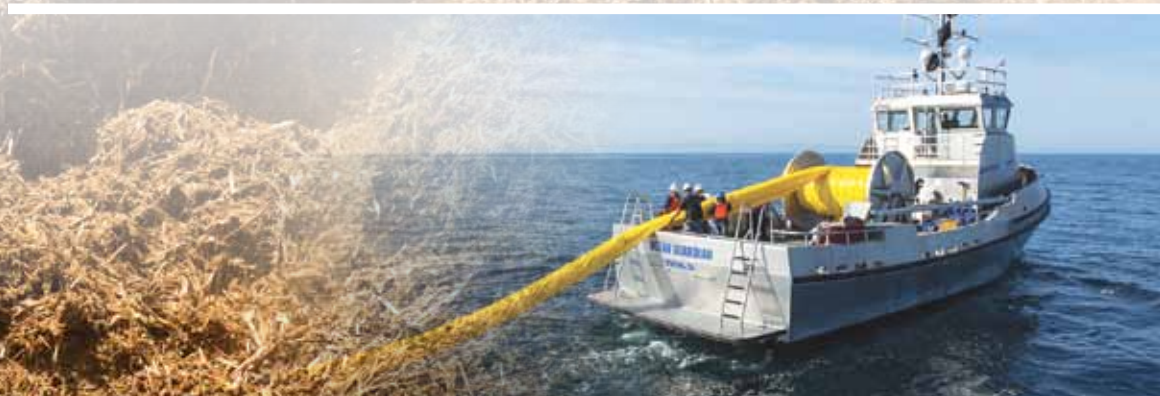
▲ Above: Ocean Guardian , one of four new 70-foot (21-meter), all-aluminum Oil Spill Recovery Vessels (OSRV) built by Rozema Boatworks for Clean Seas, a not-for-profit environmental coalition of companies operating in the Santa Barbara Channel, California, relies on twin Caterpillar 1600-hp (1193-kW) engines working through Twin Disc MGX-6599 QuickShift® marine transmissions to deliver the speed (26 knots) and agility to quickly respond to platform spills and deploy its extensive array of skimming equipment and dispersants.
