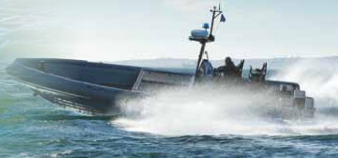
▲ Above: This 36-foot (11-meter) high-performance Rigid Inflatable Boat (RIB) built by Willard Marine, Anaheim, California, for the U.S. Navy features a Cummins 380-hp (283-kW) engine driving through a Twin Disc MG-5075SC marine transmission to power a Doen Water Jet.
