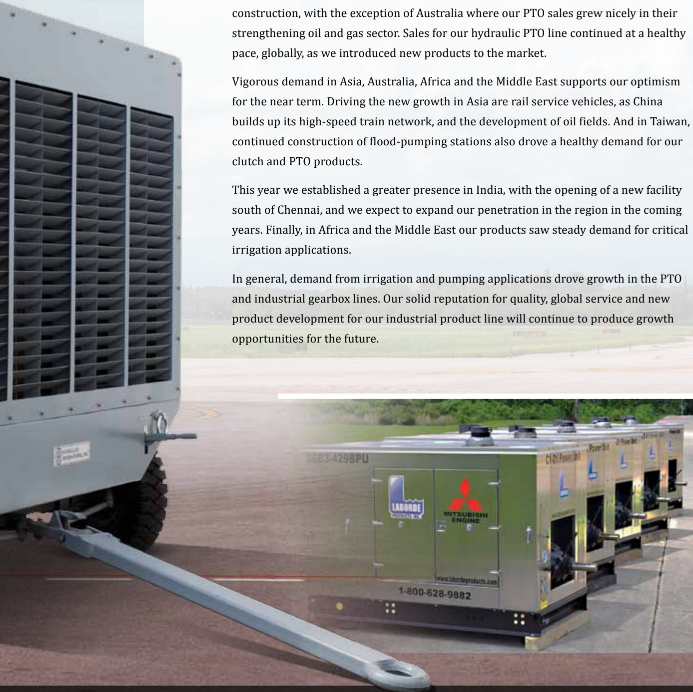
▲ Above: Laborde Products, Covington, Louisiana, manufactures specialized diesel power units such as these with 429-hp (320-kW) Mitsubishi engines working through Twin Disc SP214 PTOs and meeting Class 1, Division 1 standards for use in hazardous areas to drive pumps on 30,000-barrel (1,260,000-gallon) petroleum tank barges.
