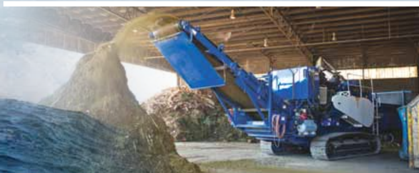
▲ Above: Powered by a Caterpillar 1150-hp (858-kW) engine working through a Twin Disc HT 600 Series Clutch, this Peterson 6710B Track Mounted Horizontal Grinder provides CST Organics with the mobility to deliver heavy-duty, high-volume grinding virtually anywhere on a job site.
