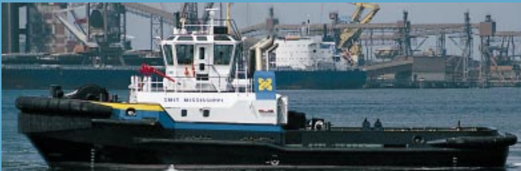
Smit International controls ship traffic in Rotterdam harbor with their fleet of 12 high-tech tugs equipped with Twin Disc MCD 3000 Marine Control Drives that permit precise maneuverability as well as engine power splitting between propulsion and fire fighting pumps.
