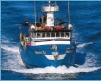
Peggy Jo, a 99' fishing boat powered by a 12-cylinder Cummins engine generating 1100 horsepower through a Twin Disc MG-5301 Marine Transmission, fishes the Bering Sea and Gulf of Alaska.
