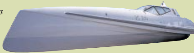
Stealthy 50' patrol boats built by FR. Lürssen Werft GmbH. & Co. in Germany for Indonesian Customs are equipped with twin 600-horsepower engines driving Twin Disc ASD-10 B1L Arneson Surface Drives through MG-5114 Marine Transmissions.
