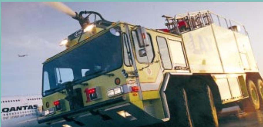
LAX International Airport has high-capacity, fast-response Aircraft Rescue and Fire Fighting (ARFF) capability with its Emergency One 8x8 Titan HPR™ equipped with a 1000-horsepower Detroit Diesel engine and Twin Disc TD-61-2619 Automatic Transmission System.
