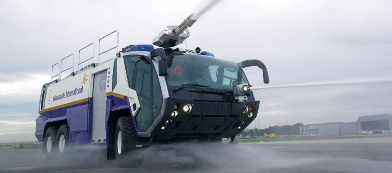
Above: Rosenbauer's Panther 6 x 6 Airport Rescue and Fire Fighting (ARFF) vehicle utilizes a TD 61-1180 transmission system for optimum acceleration to get on-scene faster and then apply "pump and roll" capability to split engine power between fire suppression equipment and precise maneuvering.
