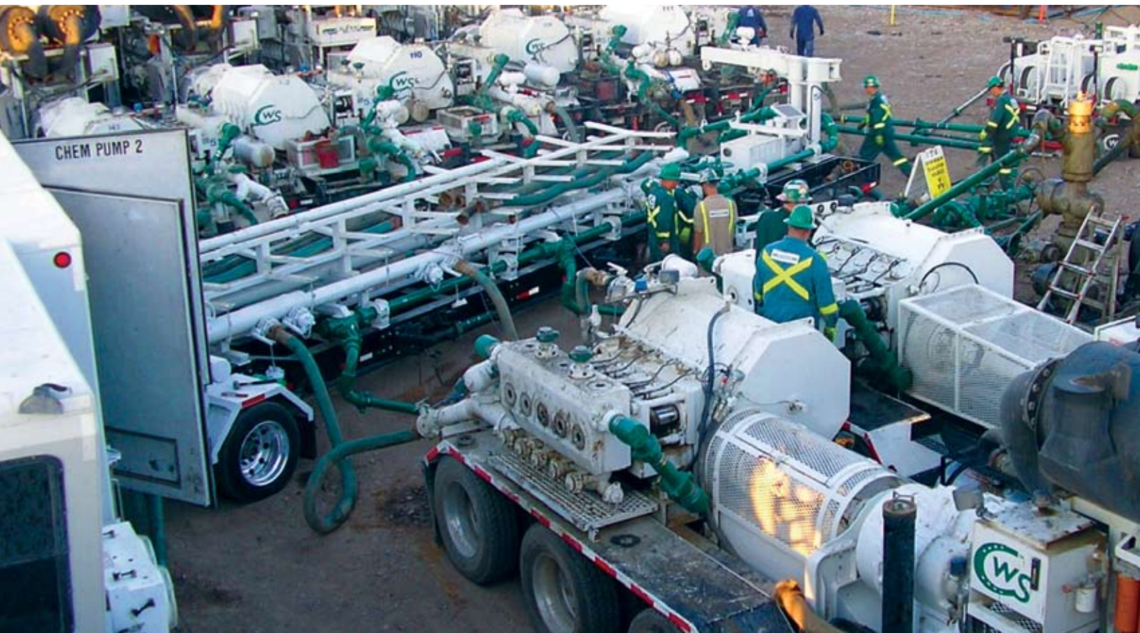
Below: At this fracturing operation in the DJ Basin near Denver, Colorado, Calfrac has seven Quintiplex frac rigs (a.k.a. "Bad Boys") using Twin Disc 8500 transmissions harnessing 2250 horsepower apiece to drive sand pumps.
