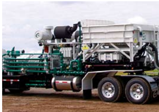
Below: At this fracturing operation in the DJ Basin near Denver, Colorado, Calfrac has seven Quintiplex frac rigs (a.k.a. "Bad Boys") using Twin Disc 8500 transmissions harnessing 2250 horsepower apiece to drive sand pumps.
