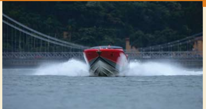
Right: Built by Power Boat Shipyard, this 52' Superboat in Sao Vicente, Brazil, achieves a top speed of 70 knots via three 440-hp (328-kW) Yanmar engines driving Arneson ASD8 Surface Drives through Twin Disc MG-5061A transmissions.
