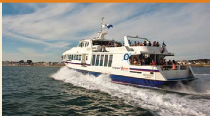
Right: Operated by Compagnie Oceane and equipped with twin Cummins 1400-hp (1044-kW) engines and Twin Disc MGX-6620SC QuickShift® transmissions with three-station EC300 controls, passenger/freight ferry Kerdonis operates from the mainland French port city of Quiberon, Brittany, to Belle Ile and Hovat.
