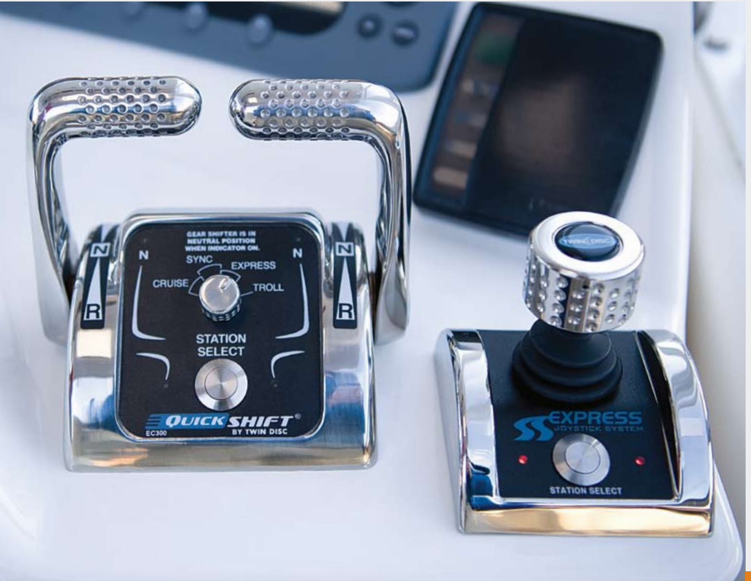
Above and left: The Twin Disc Express Joystick System (EJS), evolved from the QuickShift® transmission and EC300 controls, revolutionizes docking and slow-speed maneuvering for diesel-powered, conventional driveline boats. It gives instant access to full or incremental power in any direction, immediate yet shockless shifting from forward to reverse, and propeller control down to 50 rpm. The EJS simultaneously actuates and controls engines, transmissions and thrusters. With intuitive, easy fingertip movements the boat operator can instantaneously control all aspects of vessel direction and speed.
